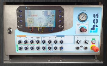
The superstructure can be controlled with the controlling panel with 9" colour intuitive display or radio remote control AUTEC.
